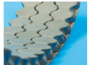
SiC DuktAr elements with steel sheet backing.
